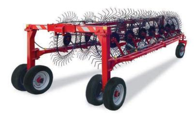
STC 14 Pull Type Wheel Rakes offer working width up to 850cm. The heavy duty frame, and wide space between wheels and tires allow customers to use this machine in wider and rough fields.
